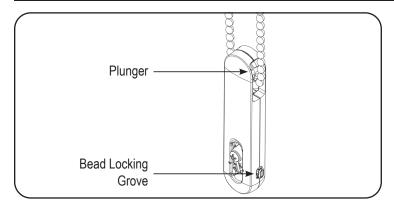
**NOTE:** For the shade to operate properly, the tensioner must be correctly mounted and secured.
